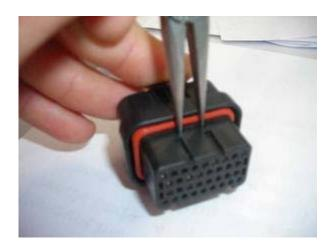
1.4.2. Using pliers, remove the plug from the ECU connector corresponding to the empty position 29 (see following image). The position of the cable is stamped on the connector itself;
