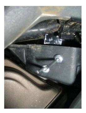
2.13. Fasten the solenoid onto the plate with the plastic clamp, with the connector facing upward.
